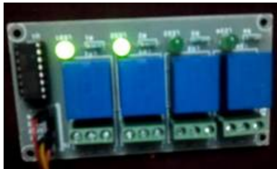
Figure 5: An electric relay board
